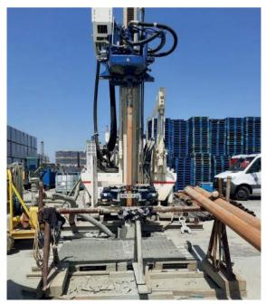
On this Mi12, the Massenza technical team used a hydraulically driven device by means of a gear motor and chain with high pull and maximum thrust of 150kN
